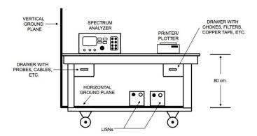
The cart can be made of wood, plastic, or fiberglass, but not metal. The cart can be rolled to wherever it is needed, and has everything required, to perform the precompliance tests as well as apply fixes to the equipment if necessary. The spectrum analyzer and a plotter, or printer (both optional), can be placed on the top of the cart. One of the two drawers can be used for the necessary precompliance test equipment, such as:
