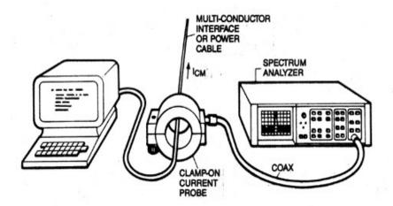
Make it a habit to measure the common-mode currents on *all* your cables! Do it early in the development process, on prototype models, while it is still easy to make a change to the product, and prior to performing final EMC compliance testing. If you fail the precompliance common-mode current test, you will also fail the radiated emission test.
