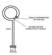
Small, shielded magnetic field loop probes are available from a number of manufacturers at very reasonable prices, a few hundred dollars or less. As an alternative to a commercial magnetic field probe a simple homemade probe can be constructed from a 50-ohm coaxial cable. One end of the cable should be formed into a 1/2 to 1 inch diameter loop with the cable center conductor soldered to the shield as shown in the figure. The shield should not be terminated on this end.
